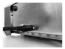
Using the power cable supplied connect the power supply to a suitable mains outlet [do not switch on the mains socket at this time].
