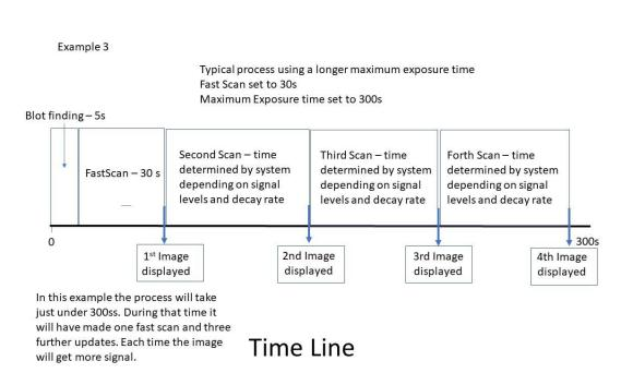
After the system has completed its process images will appear on the computer screen in the Vü software.
