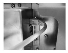
Plug the other end of the ethernet lead into a stand-alone computer. Depending on the type of computer you have you may need to use an adaptor [not supplied] to connect the ethernet lead to a suitable port.
